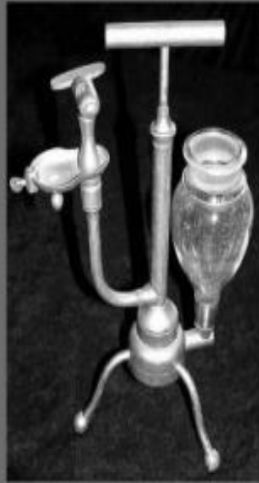
Fig. 4. The Sales-Girons "pulverisateur," which won the 1858 silver prize of the Paris Academy of Science. The pump handle draws liquid from the reservoir and forces it through an atomizer. (Courtesy of Mark Sanders, Inhalatorium.com.)
