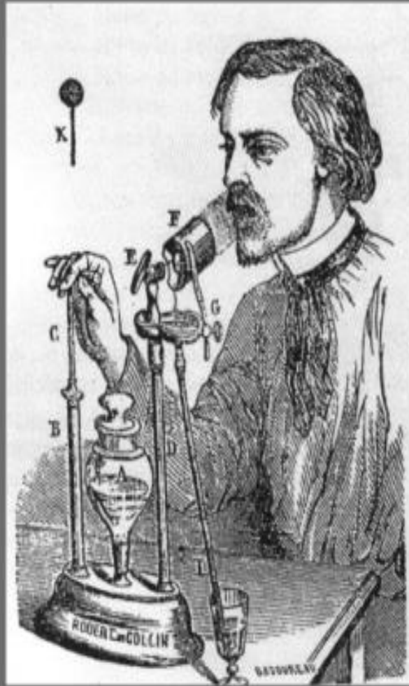
Fig. 4. The Sales-Girons "pulverisateur," which won the 1858 silver prize of the Paris Academy of Science. The pump handle draws liquid from the reservoir and forces it through an atomizer. (Courtesy of Mark Sanders, Inhalatorium.com.)
